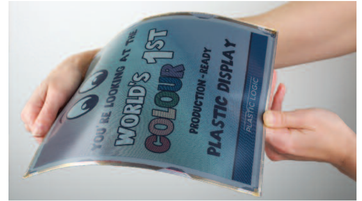
Above// Plastic Logic flexible colour plastic display (photo by Plastic Logic)
