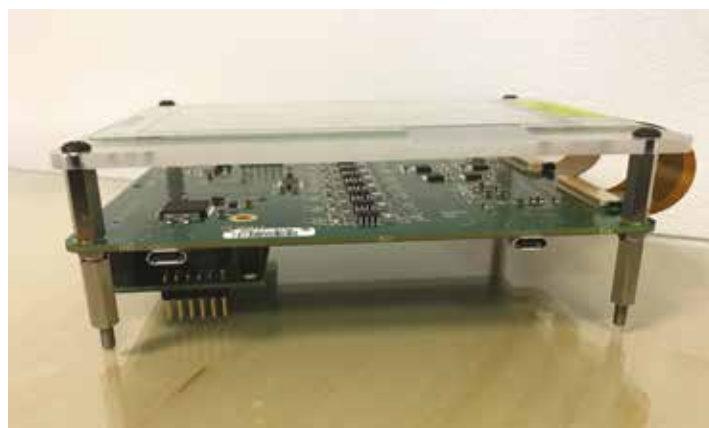
Assembled 4.3" force sensing touch platform. The thin glass force sensor is seen at the top, and built using a high volume manufacturing process for smartphone touch panels (Photo courtesy of Cambridge Touch Technologies)
